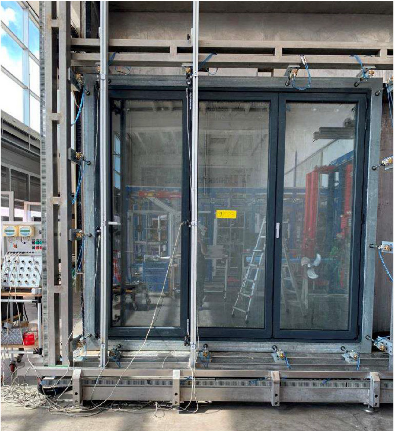
Photo 2: Sample under wind load tests
